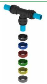
The slip-on Collet Cover shown in the illustration prevents accidental removal or tampering with tubing. Tubing can be inserted with the Collet Cover already attached to the fittings or the cover can slide into position afterwards. The cover is easily removed when required and comes in a variety of colours for colour coding.
